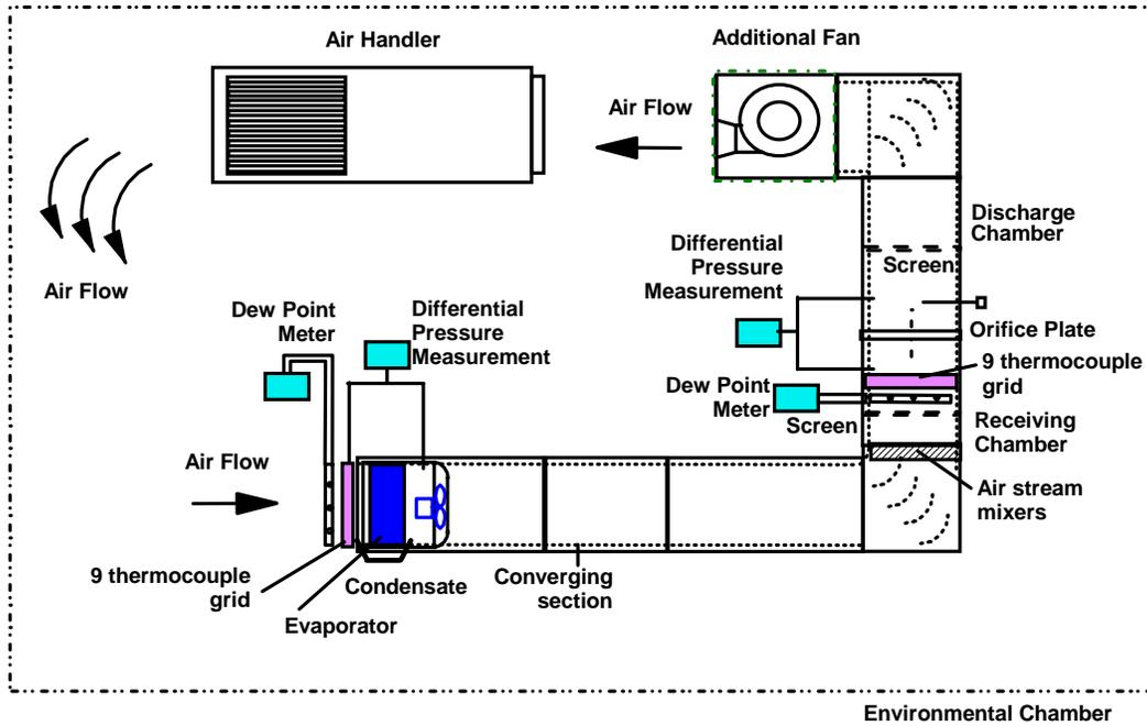
Figure 7: Test Facility for Unit Cooler
