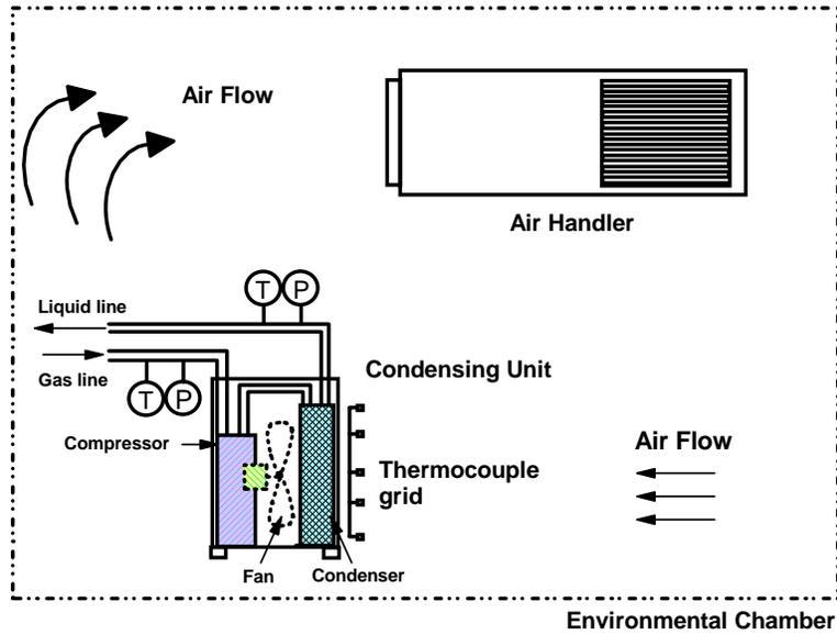
Figure 8: Test Facility for Condensing Unit
