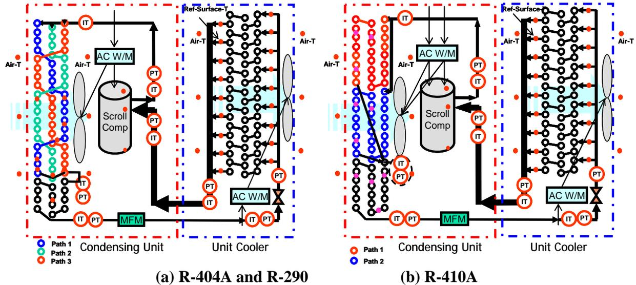
**Figure 9: Heat Exchanger Circuits and Instrumentation**
