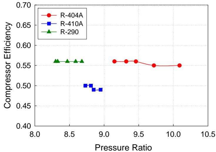
**Figure 11: Compressor Efficiency vs. Pressure Ratio**
