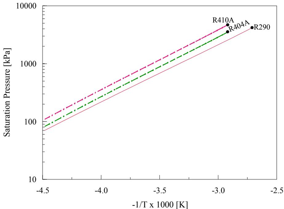
**Figure 1: Saturation Pressure of Refrigerants**
