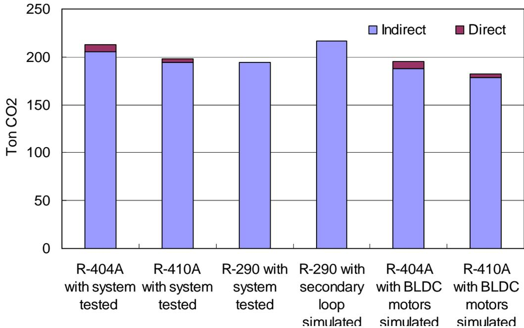
**Figure 12: Comparison of LCCP (Based on the equal compressor efficiency)**
