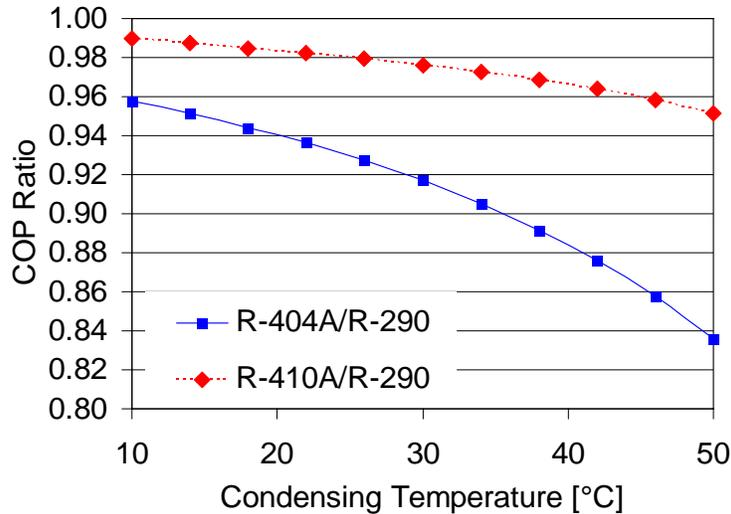
**Figure 3: Comparison of Theoretical Cycle Efficiency**
