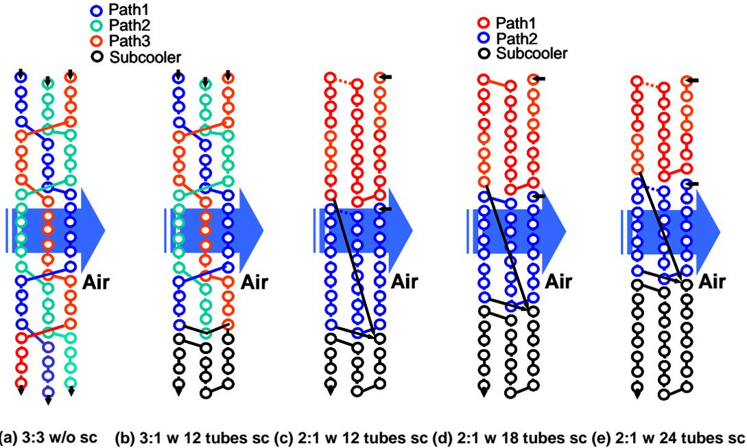
Figure 6: Condenser Circuits
